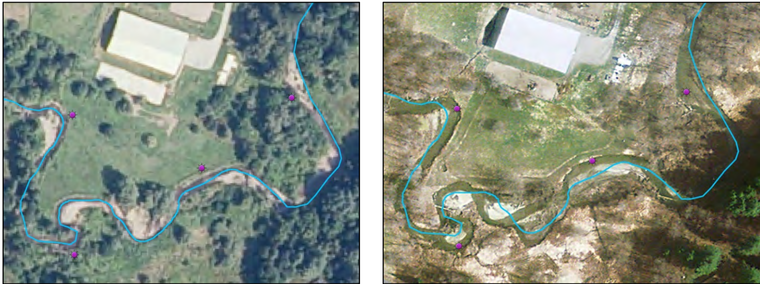
Figure 1. Side by side comparison of a location along Thatcher Brook where meander migration (purple dots) occurred likely as a result of TSI (2009 imagery on left, 2013 on right).
