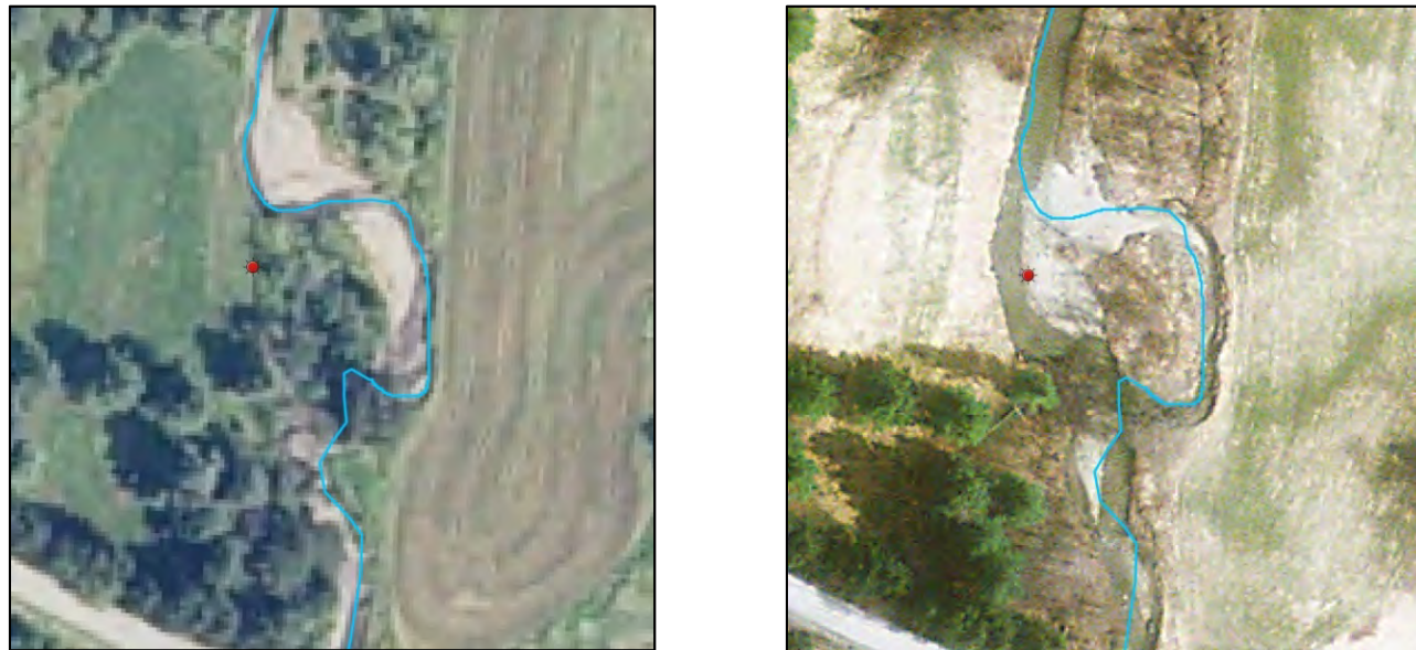
Figure 2. Side by side comparison of a location along Thatcher Brook where channel avulsion occurred as a result of TSI (2009 imagery on left, 2013 on right).
